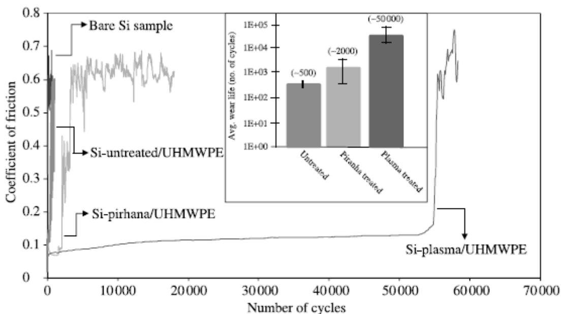
**Figure 6.** Variation of the coefficient of friction with the number of sliding cycles from typical test runs for bare Si, Si-untreated/UHMWPE, Si-piranha/UHMWPE and Si-plasma/UHMWPE samples. A normal load of 1 N and a rotational speed of 200 rpm (0.042 m/s) were used in the sliding tests. (Inset) Bar graph showing the average wear lives (in terms of number of cycles) for the three different conditions.
