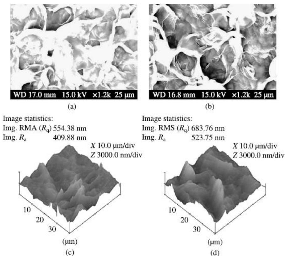
**Figure 2.** FESEM/AFM morphology of (a), (c) Si-piranha/UHMWPE and (b), (d) Si-plasma/UHMWPE films.
