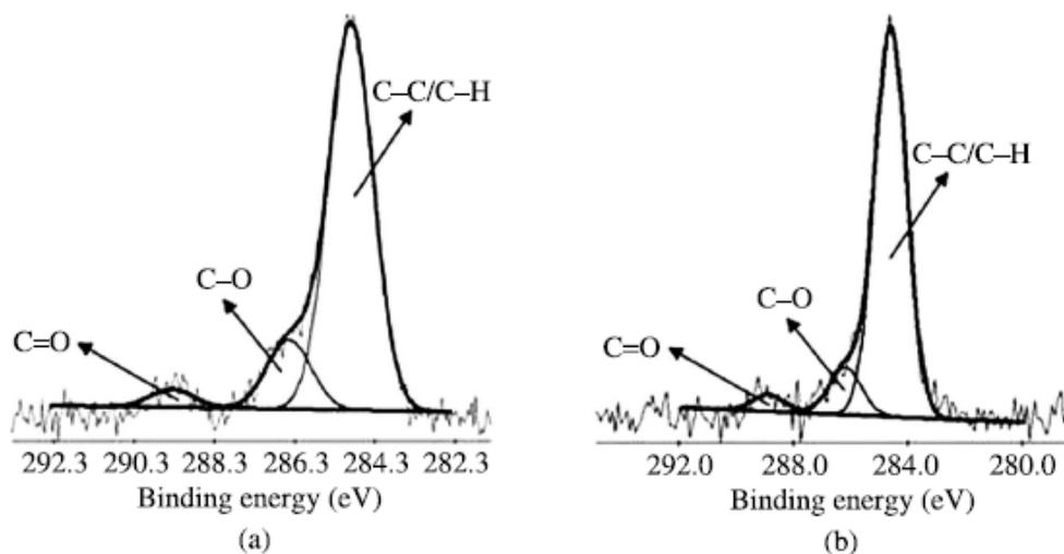
**Figure 3.** C<sub>1s</sub> core-level spectra (after curve fitting) of (a) piranha-treated Si and (b) plasma-treated Si.
