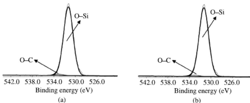
**Figure 4.** O<sub>1s</sub> core-level spectra (after curve fitting) of (a) piranha-treated Si and (b) plasma-treated Si.
