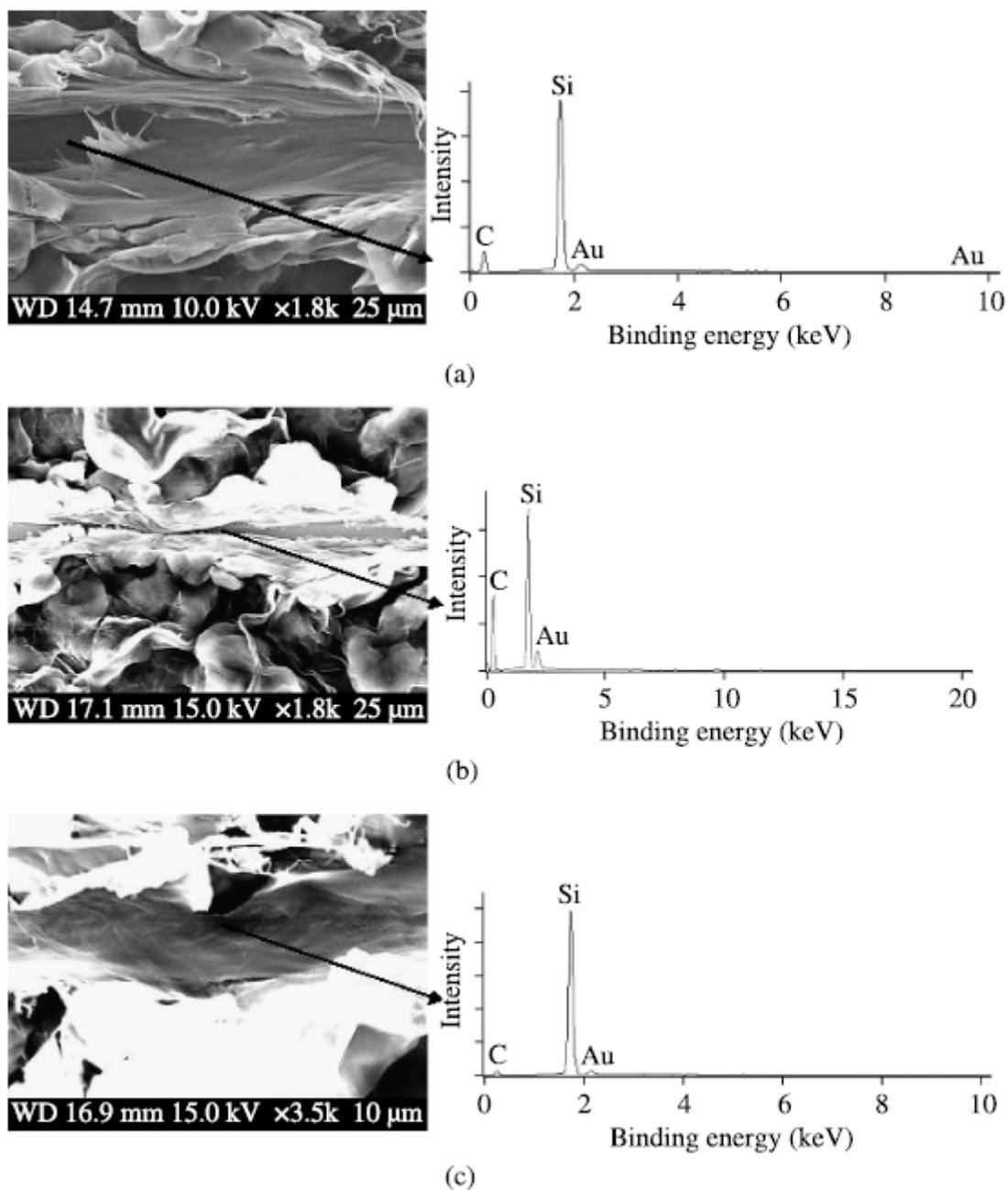
**Figure 5.** (a) FESEM morphology of a scratch made at 10 mN on Si-untreated/UHMWPE surface and EDS spectrum inside the scratch (right). (b) FESEM morphology of a scratch made at 30 mN on Si-piranha/UHMWPE surface and EDS spectrum inside the scratch (right). (c) FESEM morphology of a scratch made at 80 mN on Si-plasma/UHMWPE surface and EDS spectrum inside the scratch (right).
