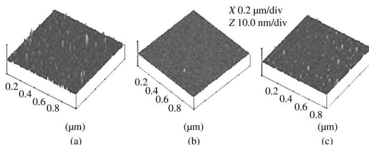
**Figure 1.** AFM topography images for (a) Si-untreated; (b) Si-piranha treated and (c) Si-plasma treated. The scan area used is  $1 \mu\text{m} \times 1 \mu\text{m}$  and the vertical scale is 10 nm.
