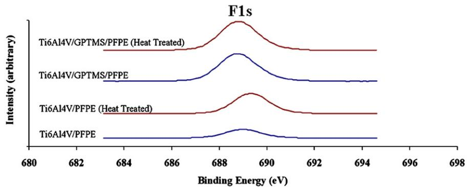
Fig. 4 – Intensities of F1s peaks for Ti6Al4V/PFPE and Ti6Al4V/GPTMS/PFPE specimens in high resolution XPS scan.
