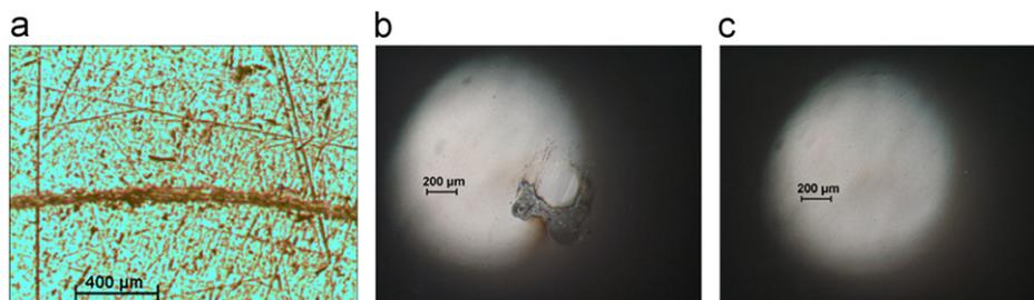
Fig. 9 – Optical micrographs of Ti6Al4V/GPTMS/PFPE specimen's wear track and counterface surface after completion of 100,000 sliding cycles. The scale bar is 400  $\mu\text{m}$  in the image (a) and is 200  $\mu\text{m}$  in the images (b) & (c). (a) Wear track, (b) counterface surface and (c) counterface surface after cleaning.
