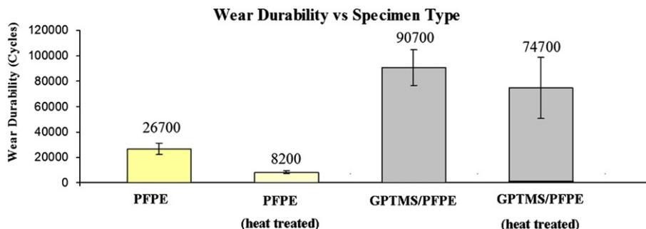
**Fig. 5 – Wear durability (number of sliding cycles before failure) of different coatings tested in the study onto Ti6Al4V substrate.**
