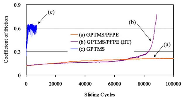
**Fig. 7 – Variation of friction coefficient as a function of the sliding cycles using Si<sub>3</sub>N<sub>4</sub> ball as the counterface (track radius: 2 mm, normal load: 0.2 N, spindle speed: 200 rpm). (a) Ti6Al4V/GPTMS/PFPE, (b) Ti6Al4V/GPTMS/PFPE (heat treated) and (c) Ti6Al4V/GPTMS.**
