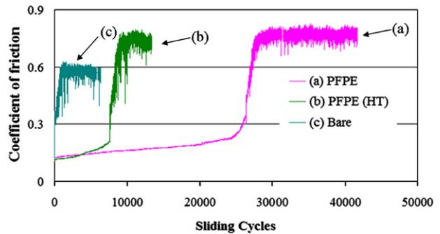
**Fig. 6 – Variation of friction coefficient as a function of the sliding cycles using Si<sub>3</sub>N<sub>4</sub> ball as the counterface (track radius: 2 mm, normal load: 0.2 N, spindle speed: 200 rpm). (a) Ti6Al4V/PFPE, (b) Ti6Al4V/PFPE (heat treated) and (c) Ti6Al4V.**
