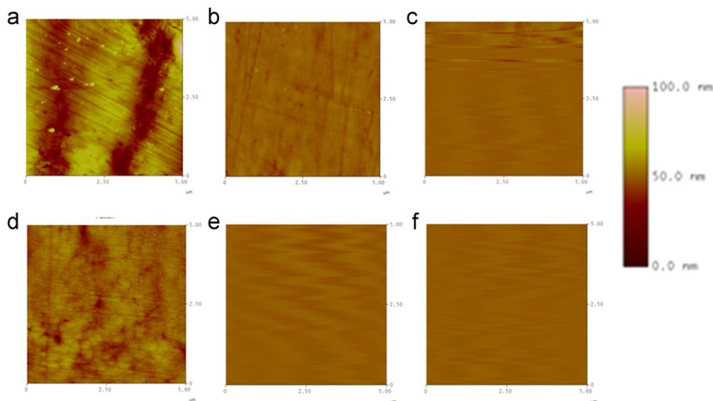
Fig. 1 – AFM imaging (scan area:  $5\ \mu\text{m} \times 5\ \mu\text{m}$ , vertical scale: 100 nm). (a) Ti6Al4V, (b) Ti6Al4V/PFPE, (c) Ti6Al4V/PFPE (heat treated), (d) Ti6Al4V/GPTMS, (e) Ti6Al4V/GPTMS/PFPE and (f) Ti6Al4V/GPTMS/PFPE (heat treated).
