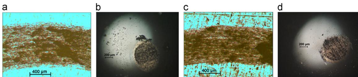
Fig. 8 – Optical micrographs of wear track and counterface surface after completion of 5000 sliding cycles. The scale bar is 400  $\mu\text{m}$  in the images (a) & (c) and is 200  $\mu\text{m}$  in the images (b) & (d). (a) Wear track (Ti6Al4V specimen), (b) counterface surface (Ti6Al4V specimen), (c) wear track (Ti6Al4V/GPTMS specimen) and (d) counterface surface (Ti6Al4V/GPTMS specimen).
