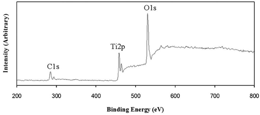
Fig. 2 – Wide scan XPS spectra of Ti6Al4V/GPTMS specimen.
