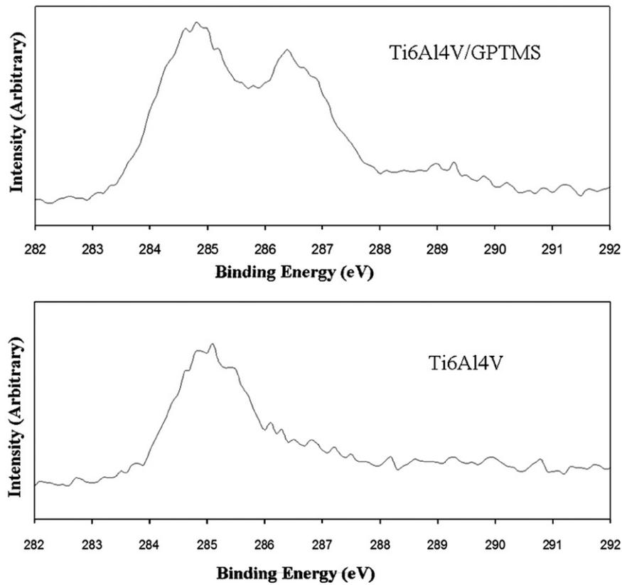
Fig. 3 – Comparison of C1s high resolution XPS scan for Ti6Al4V/GPTMS and Ti6Al4V specimens.
