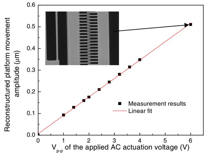
**Figure 11.** Reconstructed platform movement amplitude as a function of  $V_{p-p}$  of the applied ac actuation voltage.
