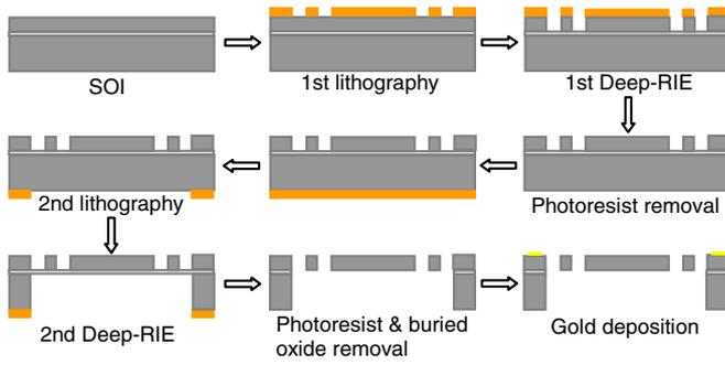
Figure 5. Fabrication process flow.
