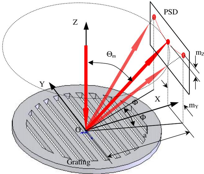
**Figure 2.** Schematic of the grating scanning-based sensing mechanism.
