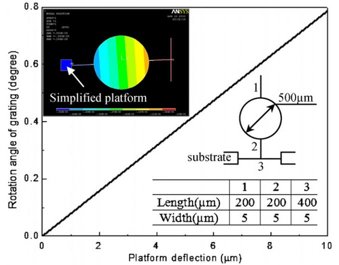
**Figure 4.** Simulation result of the grating rotation angle as a function of platform deflection. \*The structural thickness is 25 μm.
