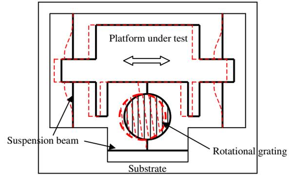
Figure 1. Schematic of the in-plane movement sensing structure.
