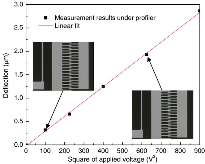
**Figure 8.** Measured platform deflections as a function of the square of the applied voltage using a Zygo profiler. (Insets are pictures of the comb-drive fingers under different statuses, in which the left fingers are fixed, while the right ones are connected to a movable platform.)
