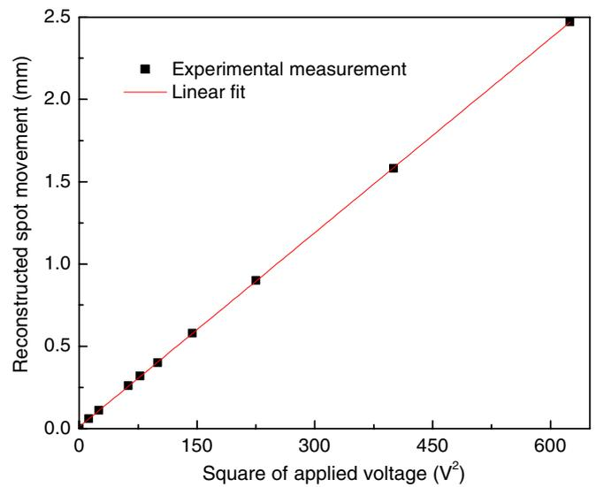
Figure 7. Reconstructed light spot movement as a function of the square of the applied voltage obtained from the experiment.
