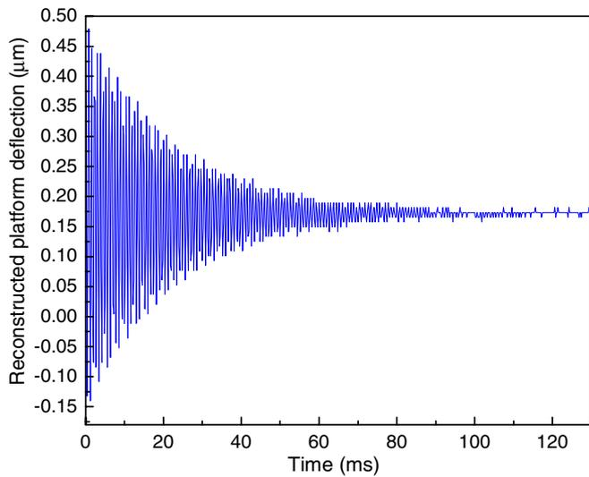
Figure 13. Reconstructed platform transient deflections.
