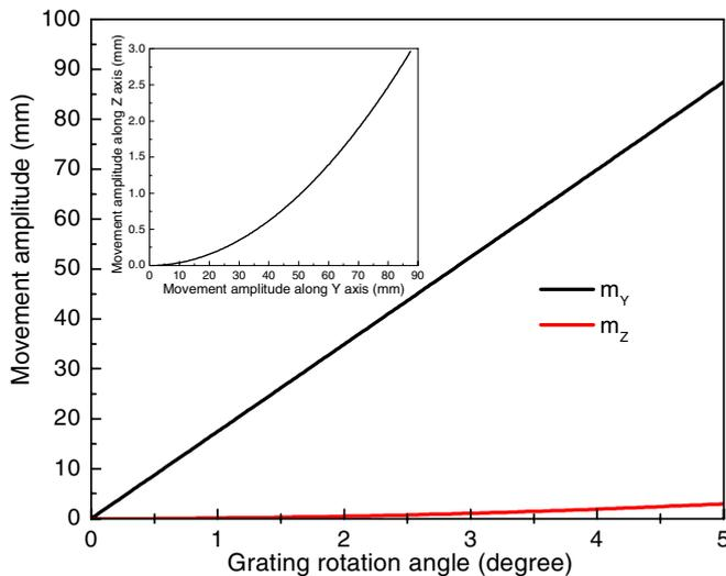
**Figure 3.** Spot movements on the PSD as a function of the grating rotation angle. Inset is the spot moving orbit on the PSD.
