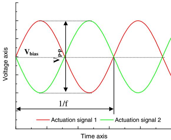
**Figure 9.** Schematic of the applied actuation signal used in the dynamic movement sensing experiment.
