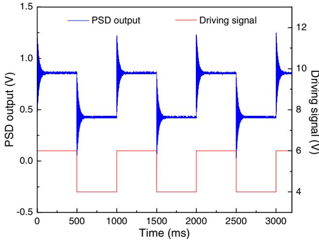
Figure 12. PSD output at a square wave actuation signal.
