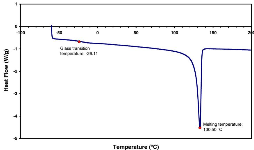
**Figure 2.** DSC data showing the glass transition and melting temperature for the polymer, UHMWPE.
