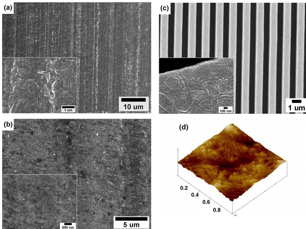
**Figure 3.** Scanning electron microscope (SEM) images of UHMWPE surfaces (a) before imprinting and after imprinting by (b) bare silicon substrate and (c)  $1\ \mu\text{m}$  gratings mould (inset shows the surface morphology of UHMWPE comprising fibrils-like structures). (d) AFM image of UHMWPE surfaces imprinted by the bare silicon substrate or  $1\ \mu\text{m}$  gratings mould.
