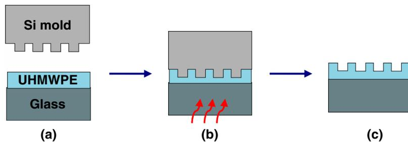
**Figure 1.** A schematic illustration of the basic NIL process. (a) Polymer is coated onto a substrate. (b) The imprint process was performed at an elevated temperature and pressure. (c) Patterned structures were transferred from the mould into the polymeric layer after de-moulding step.
