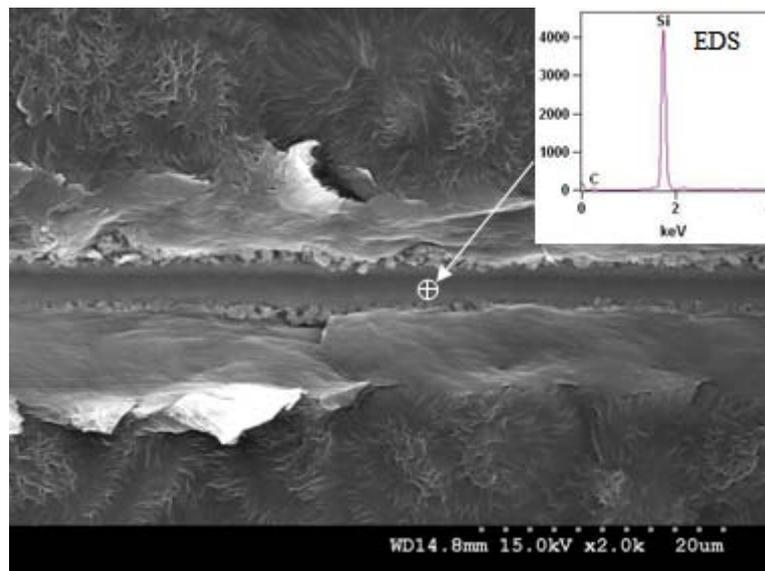
**Fig. 4** The FESEM image of a scratch on Si/DLC<sub>70</sub>/UHMWPE. The normal load during scratching was 80 mN and the scratching velocity was 0.1 mm/s.
