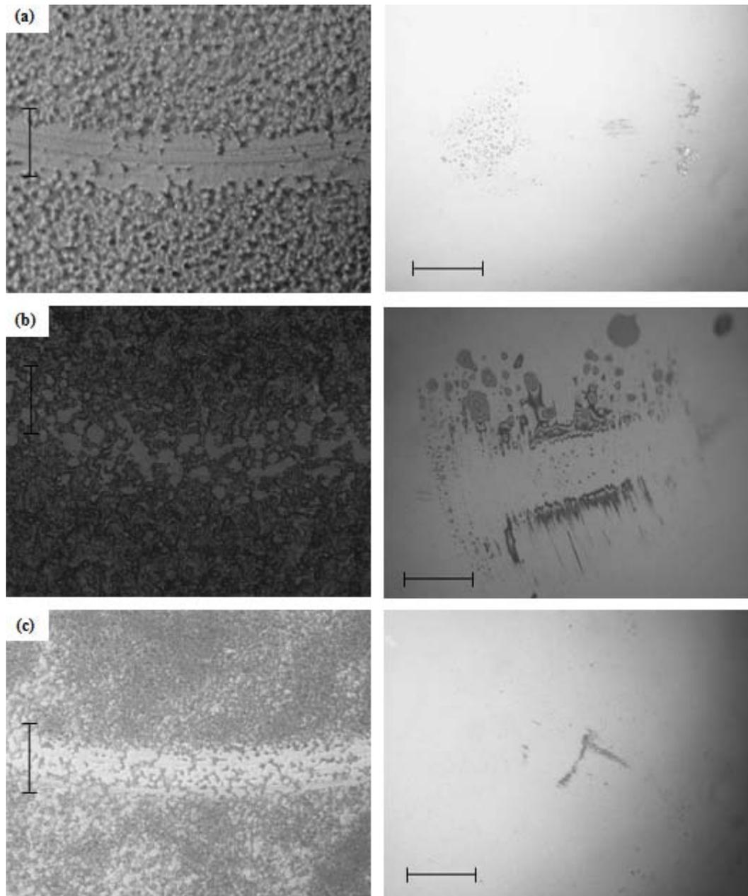
**Fig. 6** Optical microscopy images of (a) Si/TiN/UHMWPE/PFPE, (b) Si/DLC57/UHMWPE/PFPE and (c) Si/DLC70/UHMWPE/PFPE films (first column) after sliding against respective Si<sub>3</sub>N<sub>4</sub> balls (second column) for one million sliding cycles. The applied load was 70 mN and the linear sliding speed was 0.052 m/s. The vertical and horizontal scales correspond to 100  $\mu$ m.
