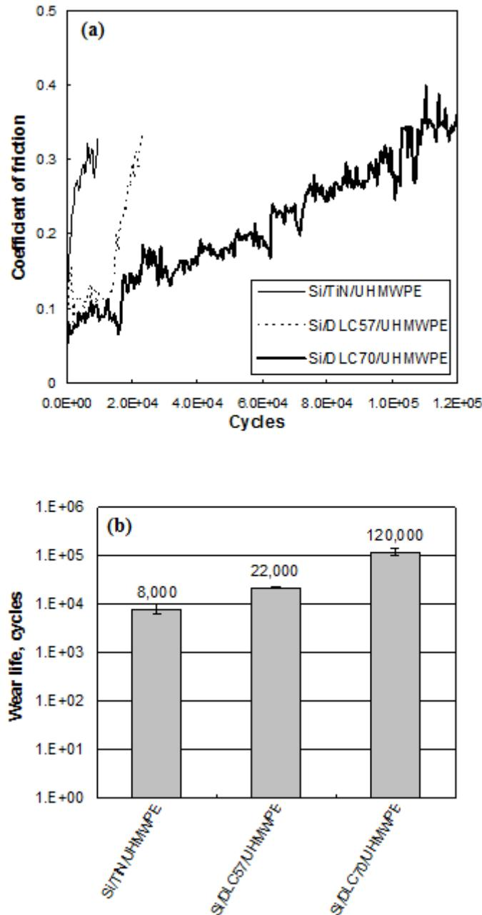
**Fig. 5** (a) Coefficient of friction and (b) wear life of Si substrate coated with different composite layers (as mentioned in the figures). The applied load was 70 mN at a rotational speed of 500 rpm (linear speed = 0.052 m/s).
