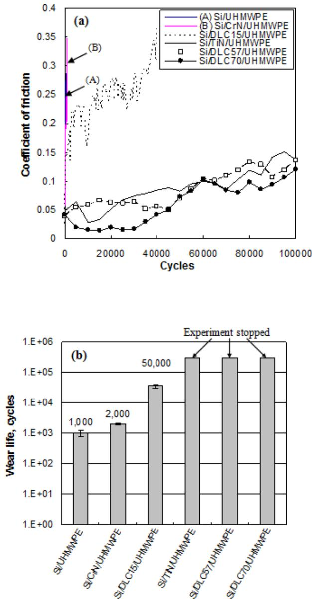
**Fig. 2** (a) Coefficient of friction and (b) wear life of Si coated with different composite films. The applied load was 40 mN and the rotational speed was 500 rpm (linear speed = 0.052 m/s).
