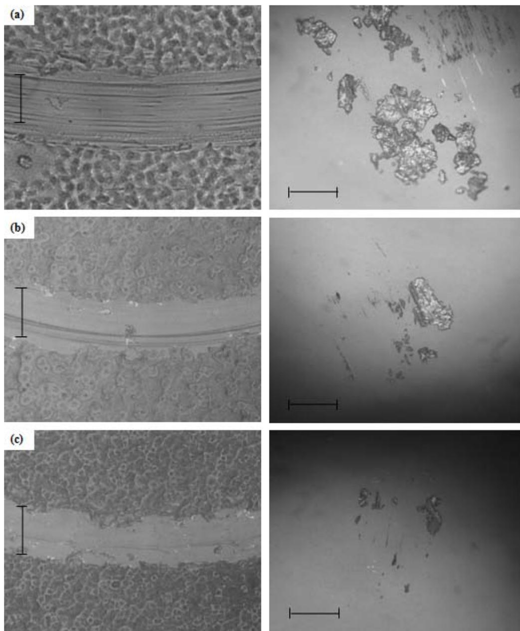
**Fig. 3** Optical microscopy images of (a) Si/TiN/UHMWPE, (b) Si/DLC57/UHMWPE and (c) Si/DLC70/UHMWPE films (first column) after sliding against respective  $\text{Si}_3\text{N}_4$  balls (second column) for 300,000 cycles where the normal load is 40 mN and the linear sliding speed is 0.052 m/s. The vertical and horizontal scales correspond to 100  $\mu\text{m}$ .
