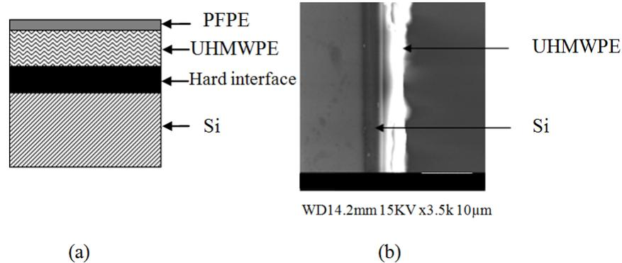
**Fig. 1** (a) Schematic (not to scale) diagram of different layers coated onto Si substrate and (b) FESEM image of the cross-sectional image of UHMWPE (white region) coated on Si substrate. The thickness of the polymer film is in the range of 4–5  $\mu\text{m}$ .
