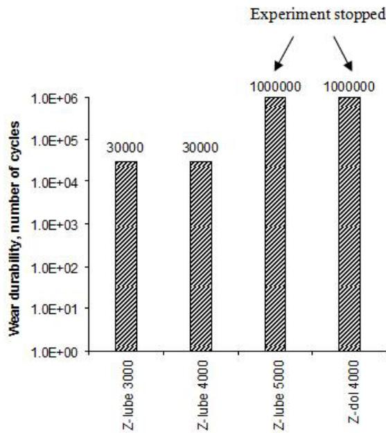
**Fig. 5** Wear durability of Z-lube (3000, 4000 & 5000 MW) and Z-dol 4000 at a normal load of 4 g and at a rotational speed of 17.33 m/s (7200 rpm).
