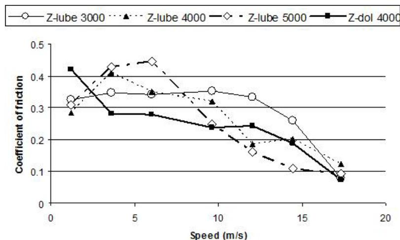
**Fig. 4** Coefficient of friction as a function of rotational speed for 4 mm Si<sub>3</sub>N<sub>4</sub> sliding against Z-lube (3000, 4000 & 5000 MW) and Z-dol 4000 for first 400 cycles.
