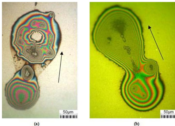
**Fig. 6** Optical microscopic image of  $\text{Si}_3\text{N}_4$  ball surfaces against (a) Z-lube 5000 and (b) Z-dol 4000 at 17.33 m/s (7200 rpm) for 10<sup>6</sup> (one million) cycles. Solid arrows show the direction of disk sliding.
