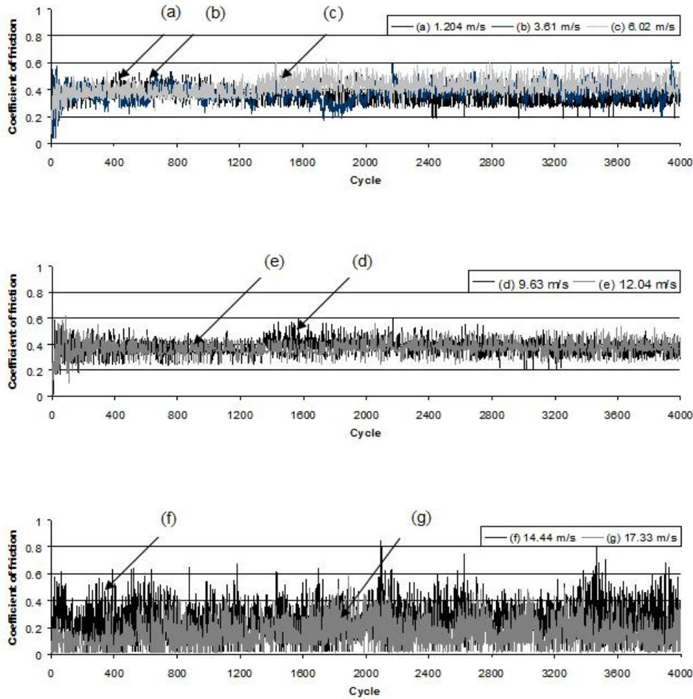
Fig. 8 Fluctuations of coefficient of friction for Z-lube 3000 at various speeds for first 4000 cycles.
