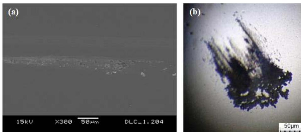
**Fig. 3** (a) SEM image of the wear track of bare disk (DLC) and (b) an optical image of Si<sub>3</sub>N<sub>4</sub> sliding ball at 1.2 m/s (500 rpm) after 400 cycles of sliding.
