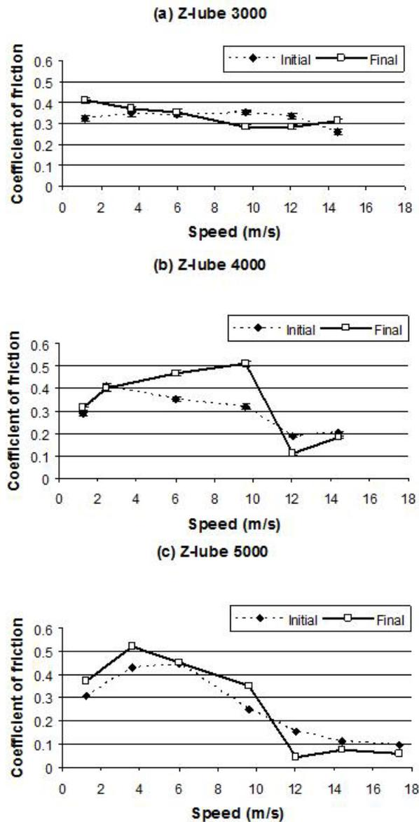
Fig. 7 Initial and final coefficients of friction as a function of rotational speeds for (a) Z-lube 3000, (b) Z-lube 4000 and (c) Z-lube 5000.
