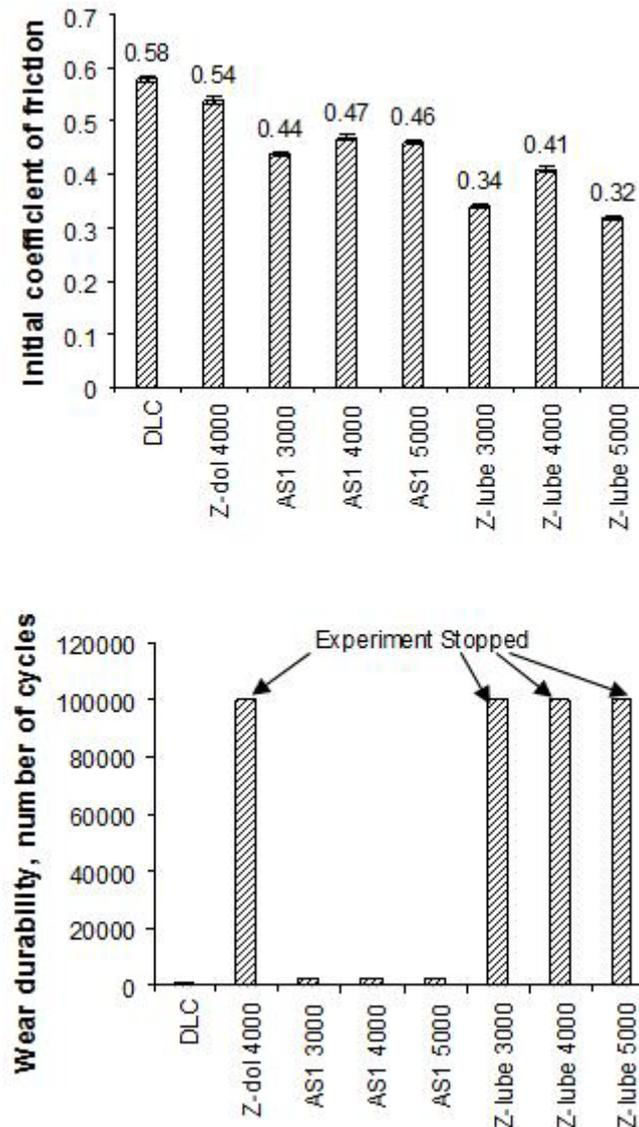
**Fig. 2** (a). Initial coefficient of friction (an average of first 400 cycles) at a normal load of 4 g and at a rotational speed of 1.2 m/s (500 rpm) for unlubricated disk and disks with different lubricants. (b). Wear durability of unlubricated disk and disks with different lubricants at a normal load of 4 g and at a rotational speed of 1.2 m/s (500 rpm).
